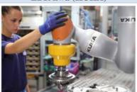
Available in 2 sizes. Integrated sensors at each joint for position control and sensitivity. Collision detection control algorithms. Image rights: KUKA AG, <a href="https://www.kuka.com/">https://www.kuka.com/</a>
