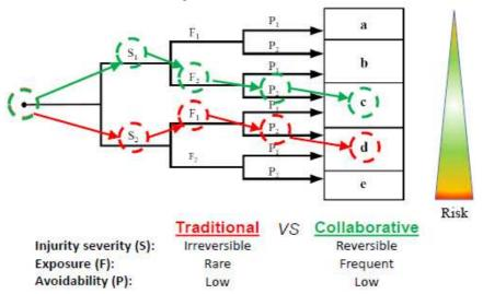
**Figure 7.3-4** The Performance Level (PL) of safety functions in control systems is based on the probability of dangerous failure per hour. An example of a comparison between traditional (PL d) and collaborative (PL c) robots from the risk assessment perspective is reported, highlighting the assessment method as per the definition of the applicable standard. *Collaborative robots can be characterized by lower PL, as the intrinsic safety guarantees higher safety levels.*
