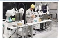
Dual-arm SCARA (Articulated Arm in the horizontal plane and end-effector with vertical motion). Easy teaching by demonstration. Extreme repeatability. <a href="https://robotics.kawasaki.com/">https://robotics.kawasaki.com/</a>
