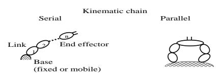
Figure 7.2-3 Example of serial and parallel kinematic chains [4].
