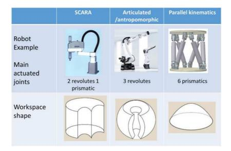
Figure 7.2-5 Main categories of mechanical structures of industrial robots.
