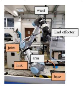
Figure 7.2-1 Robot main components.
