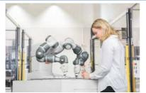
Multi-purpose end-effector: vacuum and servo grippers, camera. Padded redundant arms. Collaborative assemblies, inspection and packaging.
