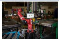
Power and force limited compliant arms (elastic actuators, sensors). Force sensors in each joint. Cameras in the wrists and in the head.
