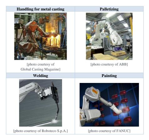
**Figure 7.2-6** Examples of applications of articulated robots. Image rights: Global Casting Magazine, ABB, Roboteco S.p.A., FANUC.
