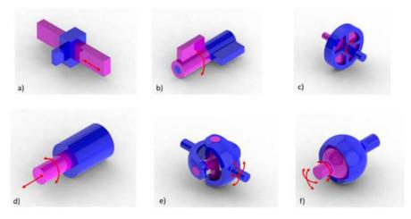
**Figure 7.2-2** Typical joints used in robotics: a) prismatic (translation along one direction), b) and c) rotoidal (hinge, rotation about one axis), d) cylindrical (rotation and translation) e) cardanic (rotation about two orthogonal axes), f) spherical (rotation about 3 axes) [4]. Image rights: Authors.
