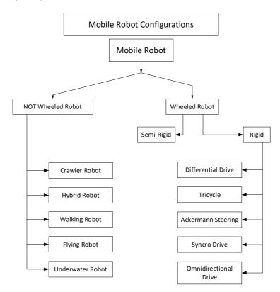
Figure 7.4-2 Classification of Mobile Robots.
