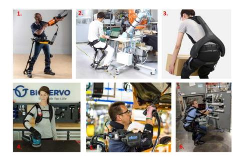
Figure 7.3-2 Exoskeletons for industrial use: 1. Fortis by Lockheed Martin Corporation (courtesy of Lockheed Martin), 2. Noonee "Chairless Chair" (courtesy of Noonee), 3. Powered Wear ATOUN MODEL Y (courtesy of ATOUN), 4. BIOSERVO Ironhand powered glove (courtesy of Bioservo Technologies AB), 5. ©EksoVest by Ekso Bionics upper body exoskeleton, 6. MAX© - Modular Agile eXoskeleton by suitX©.
