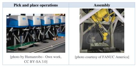
**Figure 7.2-9** Examples of applications of parallel robots. Image rights: Humanrobo, FANUC America.
