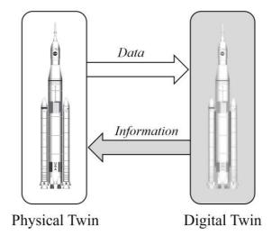
**Figure 6.1-1** The digital twin is the virtual counterpart to the physical twin, and is used to better understand complex systems such as manufacturing lines or rockets. Data collected with sensors in the physical twin inform the digital twin and
