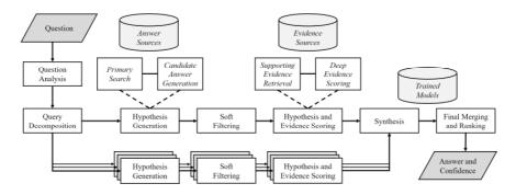
**Figure 6.4-2** IBM's Watson used advanced natural language processing to analyse a question's meaning, and then draws upon a vast database of information to hypothesis answers and weigh them up with answers. Watson may be at the cutting edge of DSS systems, but the techniques used are increasingly common in commercial solutions.
