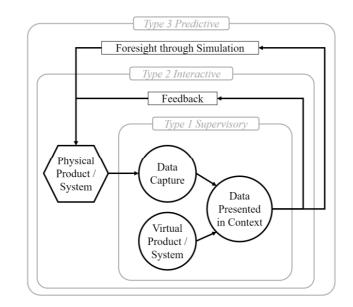
Figure 6.3-2 The types of digital twins are layered on top of one another, according to the AMRC classification [15].
